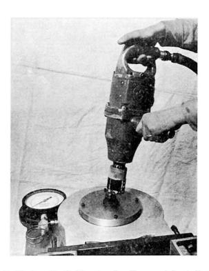
Fig. 3. Hydraulic Calibrator for Torqued Installation.
