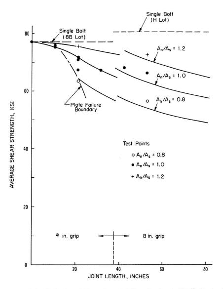
Fig. 1. Summary of Analytical and Experimental Results for A 325 Bolts in A 440 Steel Joints.
