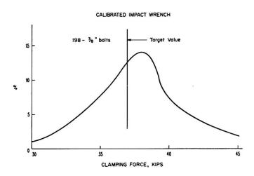
Fig. 2. Histrogram of Internal Bolt Tension.
