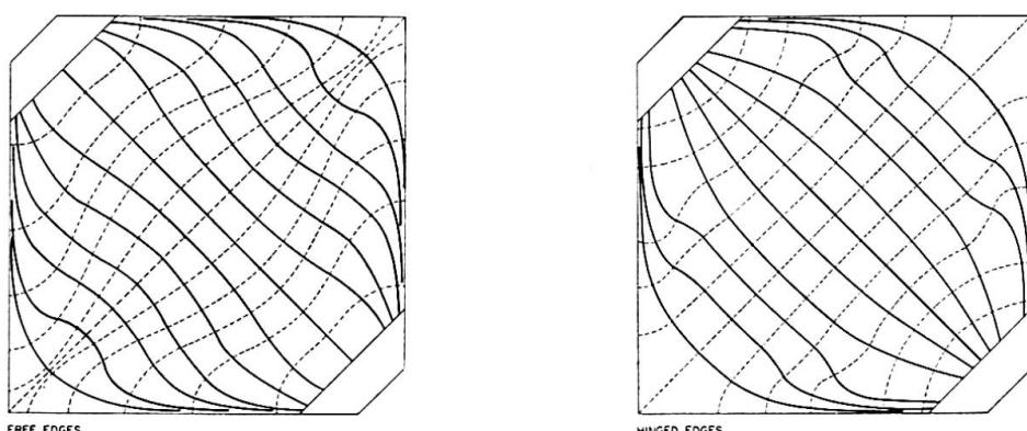
Fig. 5. Isostatics of Membrane Stresses.
