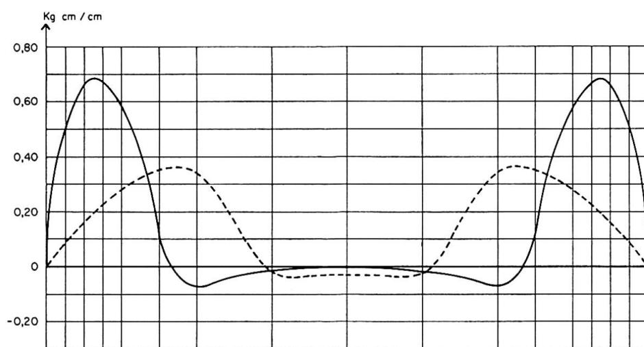
Fig. 6. Bending Moments along the Middle. Straight Generator.
