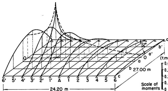
Fig. 8. Bending moments influence surface in beam 3' section 0—0'.
