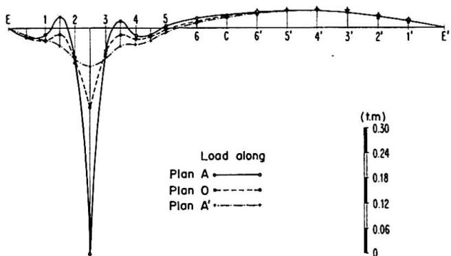
Fig. 12a. Moments in section  $S_{2-3}$  of deck beam  $A$ .
