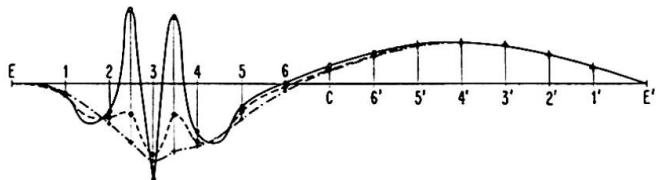
Fig. 12b. Moments in section  $S_3$  of deck beam  $A$ .
