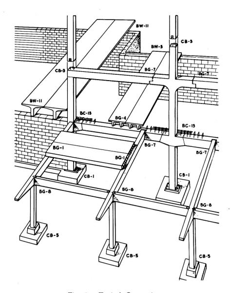
Fig. 8 - Typical Connections.
