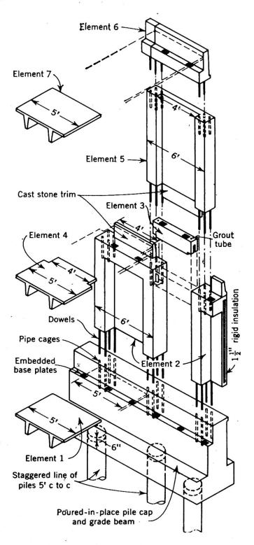
Fig. 9 - Assembly of Prefabricated Elements for Two-Story Barracks Building. Architect and Engineer: George M. Ewing Co. (Illustration courtesy "Civil Engineering").
