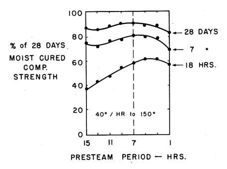
Fig. 6 - Strength Development Under Steam Curing.
