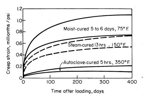
Fig. 7 - Effect of Curing on Creep of Concrete.
