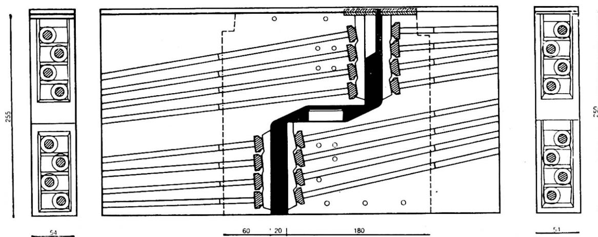
Fig. 8.4 - Details of hinge and cable-anchorage.
