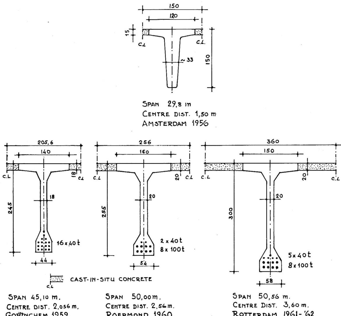
Fig. 5.3 - Sections of post-tensioned T-beams for bridges.
