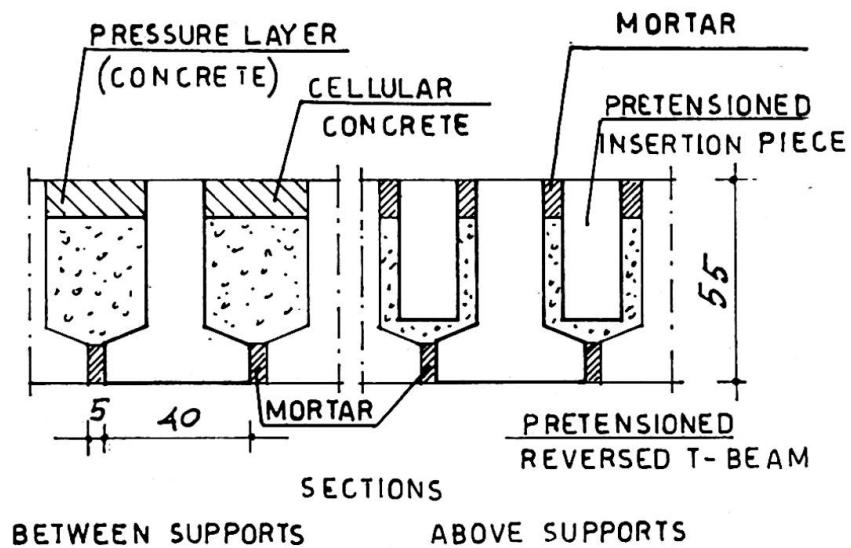
Fig. 5.1 - Composite viaduct in Highway 4A; continuity connection.
