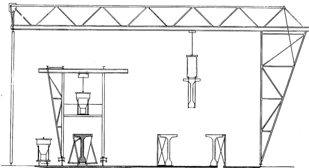
Fig. 8.7 - Casting and transportation of intermediate beams.
