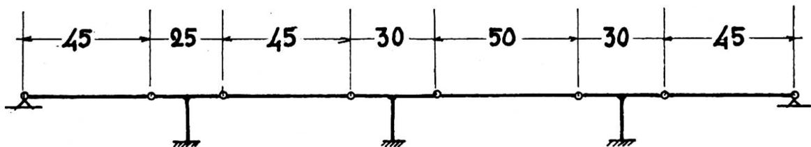
Fig. 8.3 - Statical system of the bridge.
