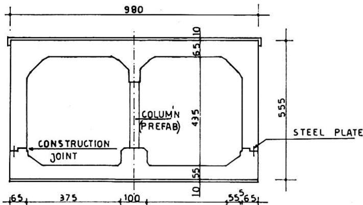
Fig. 10.1 - Cross-section of subway tunnel element Rotterdam.
