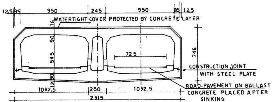
Fig. 10.2 - Cross-section of highway tunnel element Amsterdam.
