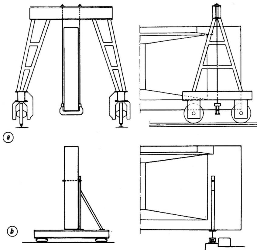
Fig. 4.4 - Longitudinal and transverse transport of bridge beams.
