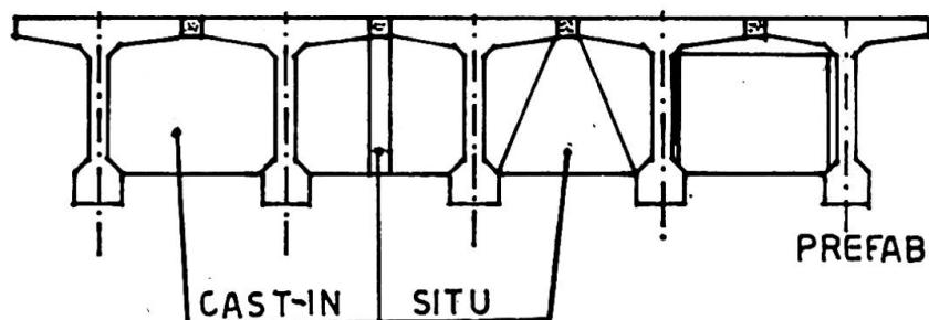
Fig. 5.5 - Execution of cross-beams.
