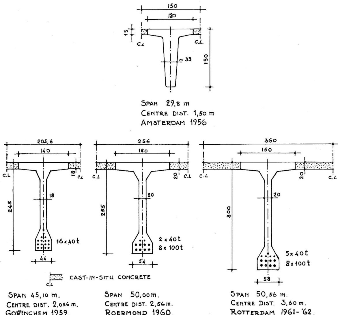
Fig. 5.3 - Sections of post-tensioned T-beams for bridges.
