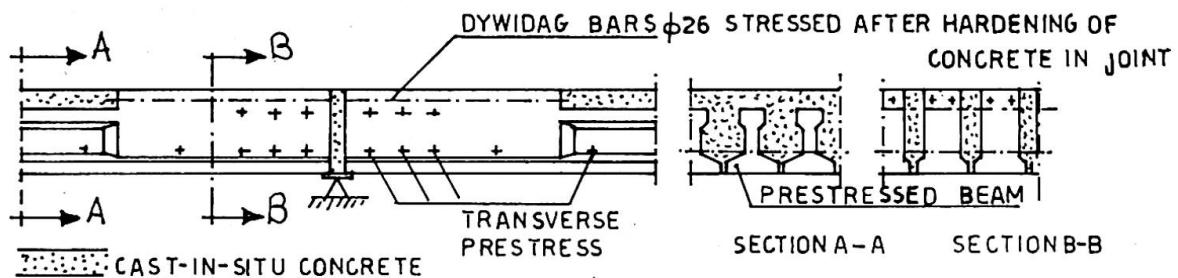
Fig. 5.2 - Continuity connection of a composite bridge.
