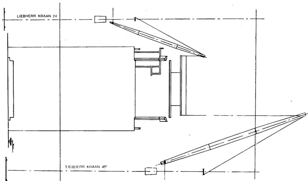
Fig. 7.4 - Placing the cylindrical shell-halves on the roof of the canteen.
