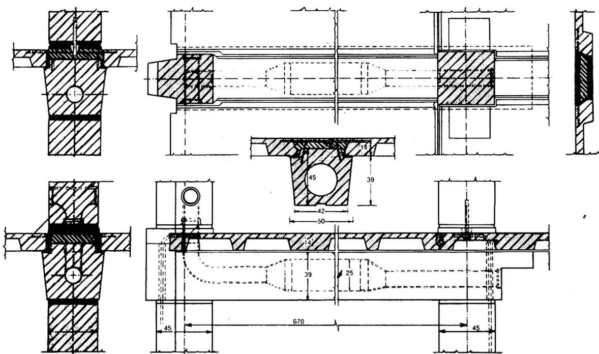
Fig. 6.5 - Connection of cross-beams, columns and floor beams.
