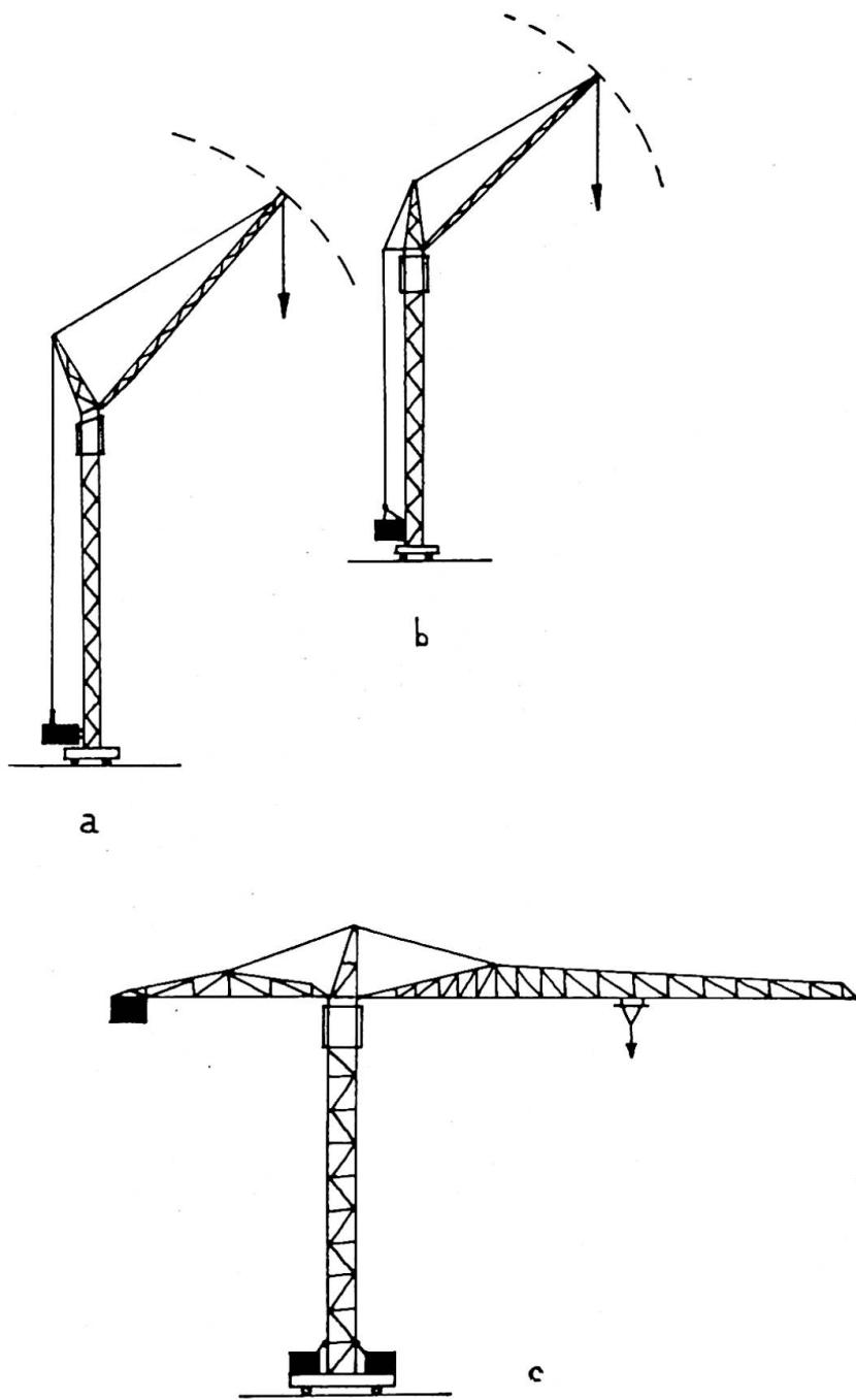
Fig. 4.1: a, b, c - Types of building cranes used the Netherlands (tower-crane).
