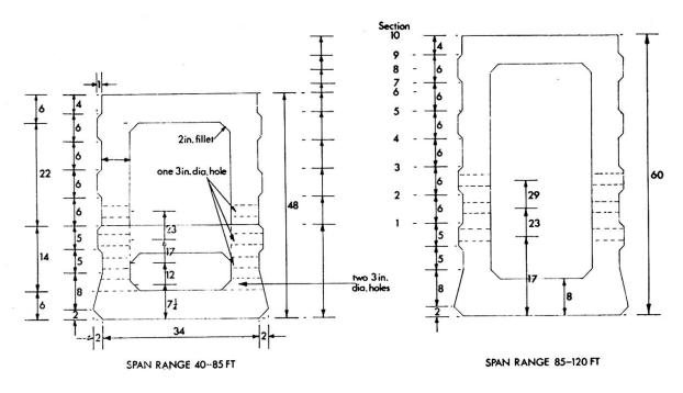
Fig. 10 - Standard box sections for bridges of span 40-120 ft.
