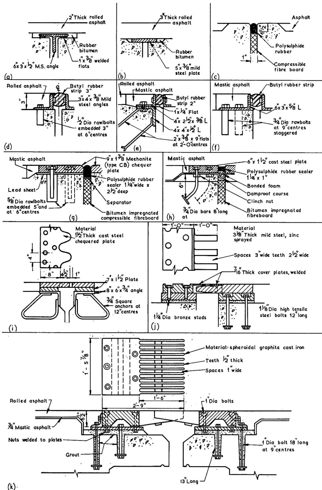
Fig. 3. Examples of joints.
