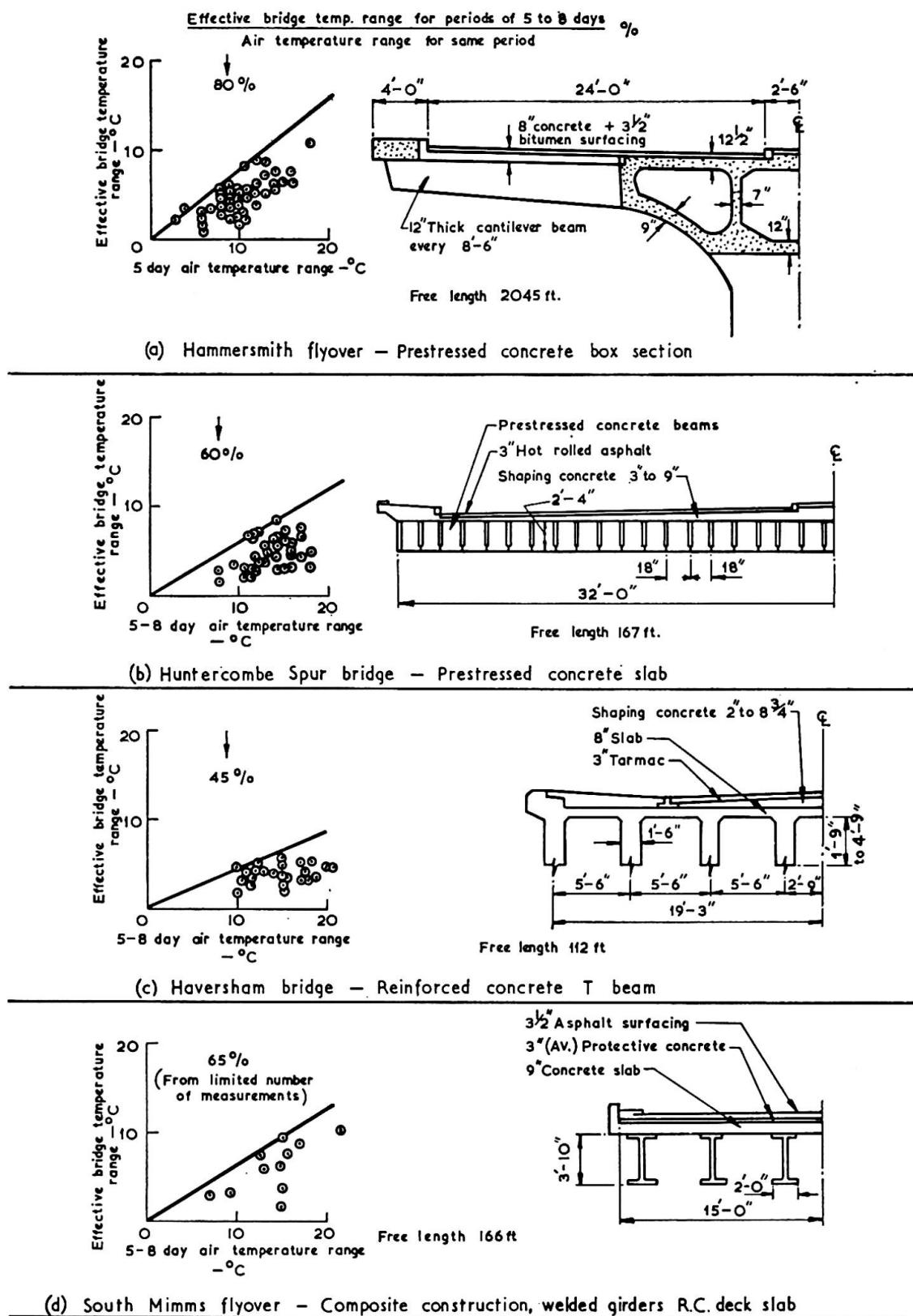
Fig. 2. Comparison of 5 to 8 day air temperature ranges with the 5 to 8 day effective bridge temperatures for various bridges.
