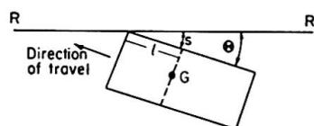
Fig. 5. Glancing impact of vehicle with rigid barrier.
