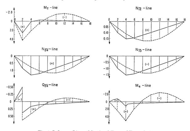
Fig. 4. Influence Lines of Sectional Force of Example 1.
