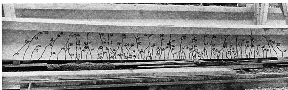
Fig. 11. Crack Distribution in the Non-Grouted T-Beam with Supplementary Mild Steel (TM).
