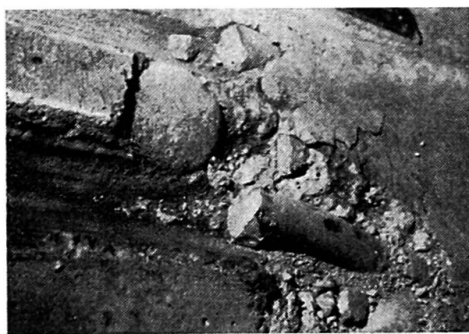
Fig. 5. The Fatigue Rupture of the Connector. The Picture Shows the Concrete Slab, Upside Down, with the Connector Ends, After Failure.
