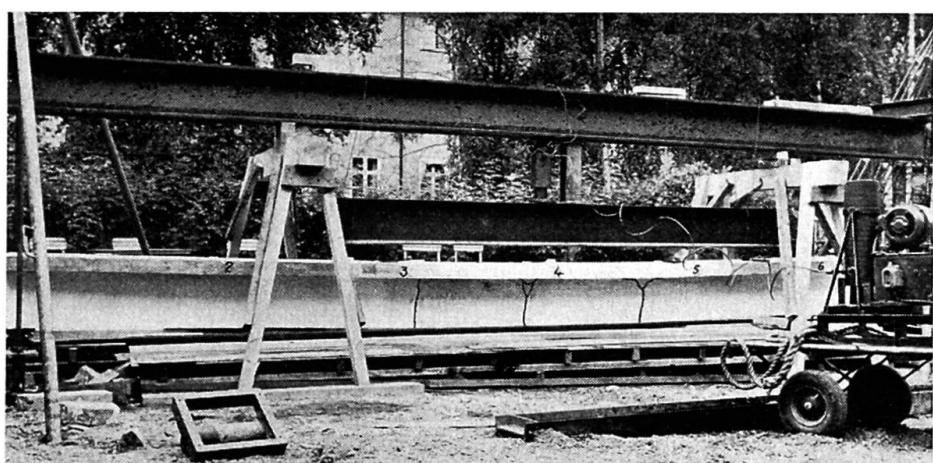
Fig. 9. Crack Distribution in the Non-Grouted T-Beam (T).
