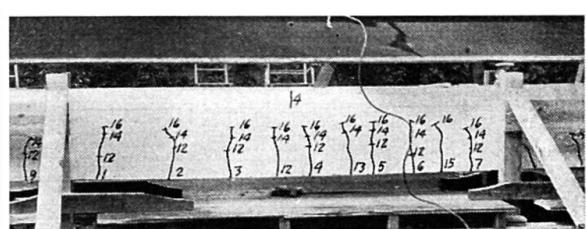
Fig. 13. Crack Distribution in the Grouted R-Beam (RI).
