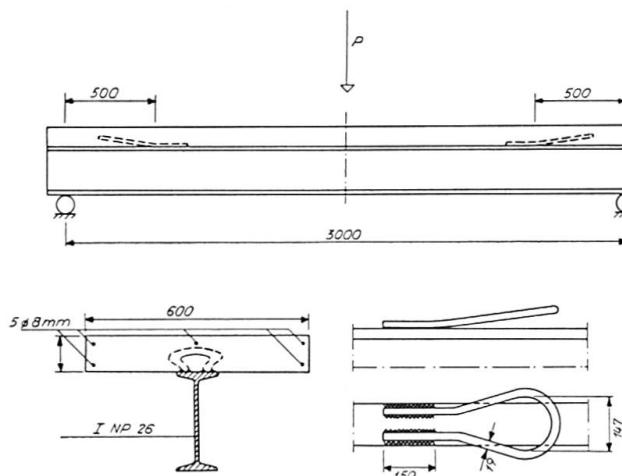
Fig. 1. Test Beams No. 1 and 2, Subjected to Positive Moment. Dimensions in mm.
