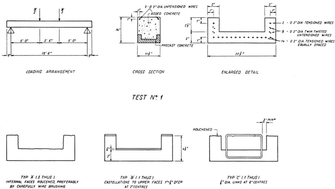
Fig. 3. Cube Strength at Transfer 7500 lbs./Squ. in. Initial Tensioning Force 2.2 Tons/Wire.
