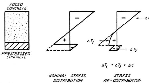
Fig. 2. Stress Re-distribution in Prestressed Composite Beams.
