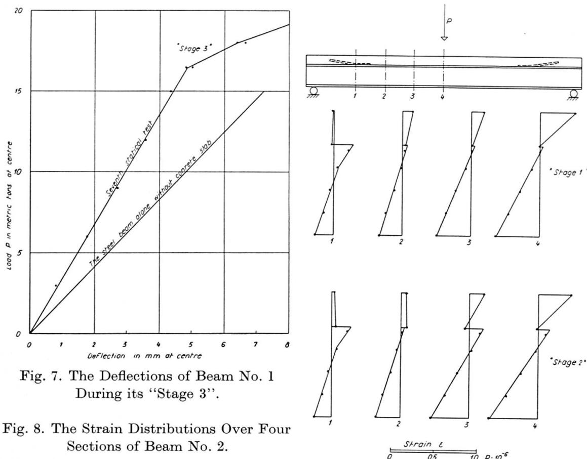
Fig. 7. The Deflections of Beam No. 1 During its "Stage 3".
