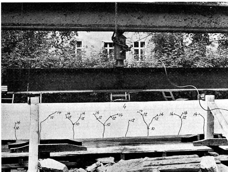
Fig. 10. Crack Distribution in the Non-Grouted R-Beam (R).
