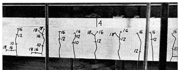
Fig. 12. Crack-Distribution in the Grouted T-Beam (TJ).
