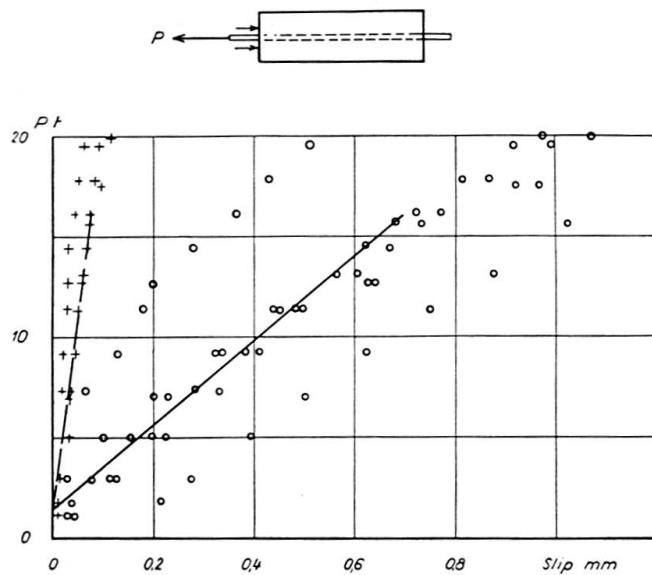
Fig. 1. Typical Result of the Pull-out Tests.
