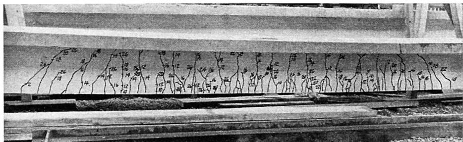
Fig. 11. Crack Distribution in the Non-Grouted T-Beam with Supplementary Mild Steel (TM).
