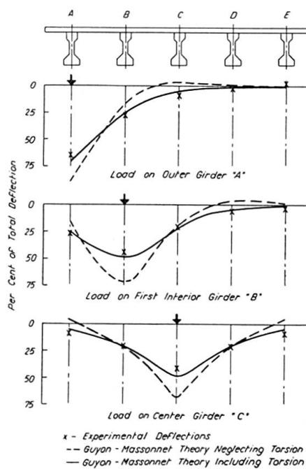
Fig. 13. Concentrated Load Tests — Series 3. Lateral Distribution of Deflections — Load at Midspan.
