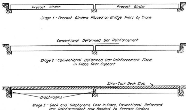
Fig. 1. Sequence of Construction of Continuous Precast Bridge.
