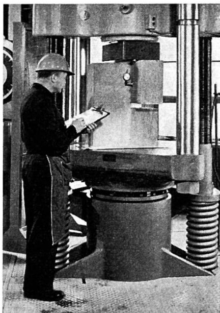
Fig. 5. Horizontal Shear Test using "Push-Off" Specimen.
