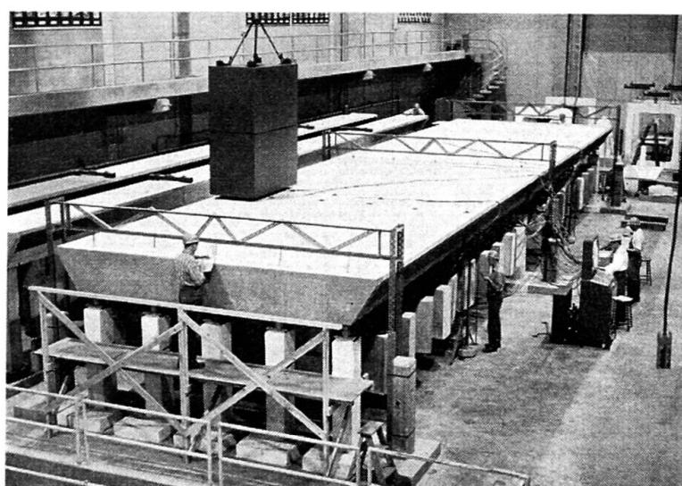
Fig. 12. Influence Surface Test of Half-Scale Highway Bridge.
