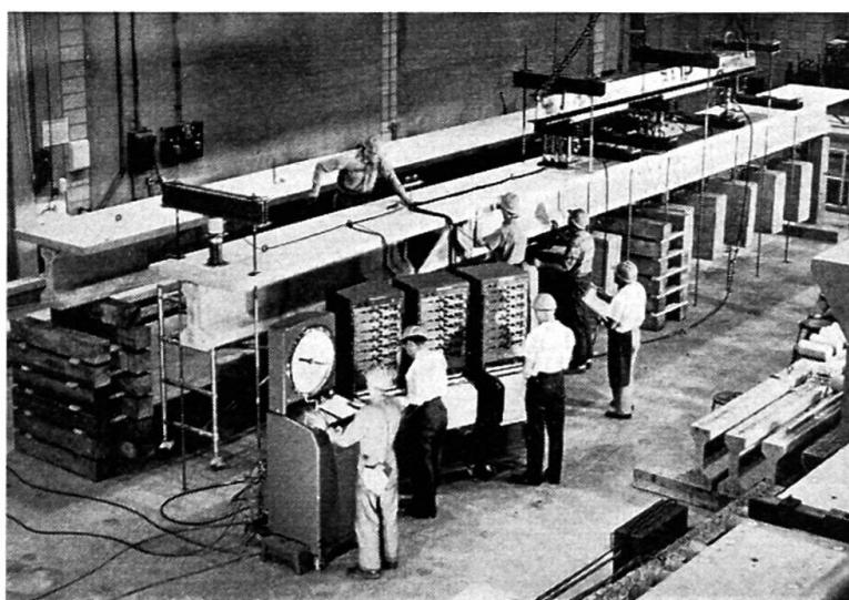
Fig. 9. Shear Test of Composite Prestressed Girder.
