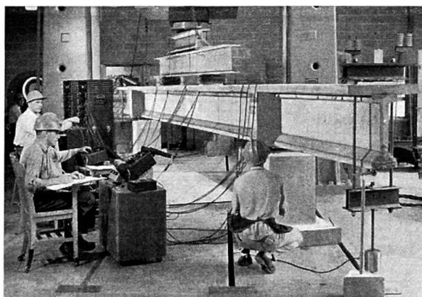
Fig. 4. Test of Continuous Girder from Group III.
