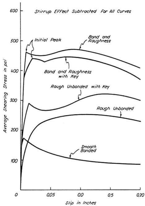
Fig. 6. Typical Shear-Slip Curves for "Push-Off" Tests.
