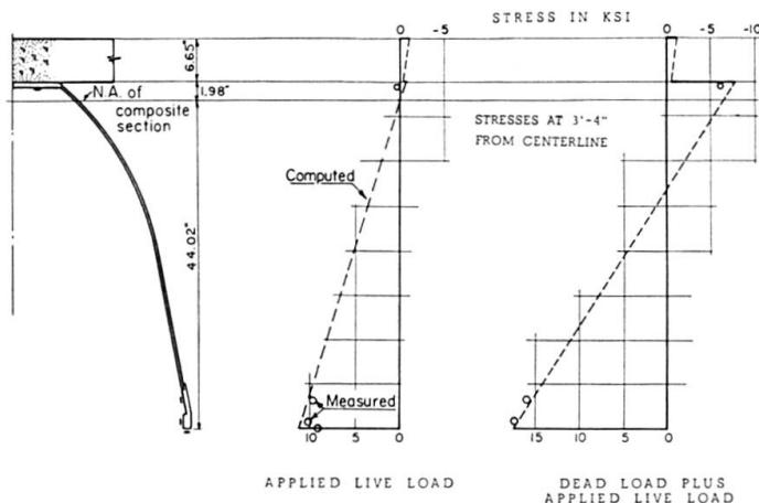
Fig. 5. Stresses at Two Times Design Moment.
