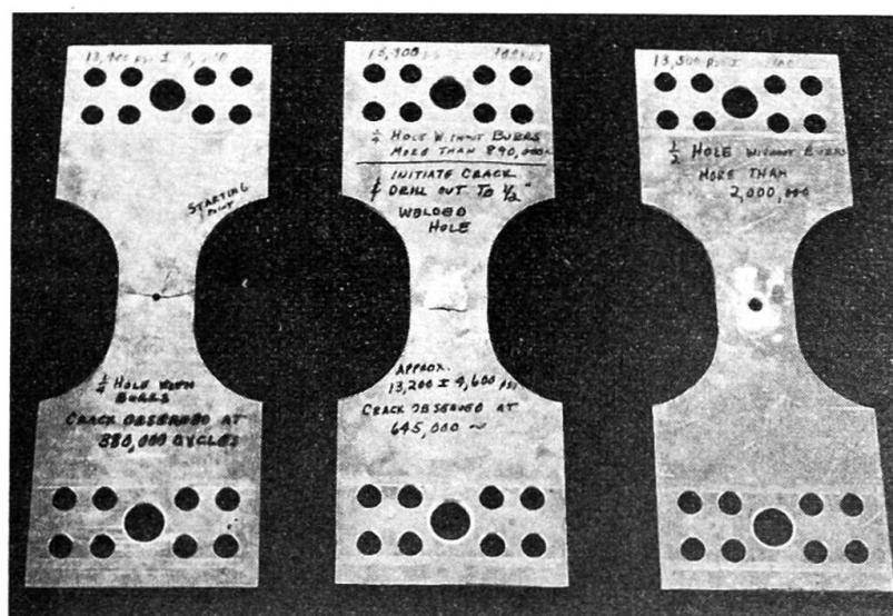
Fig. 9. Fatigue Specimens.
