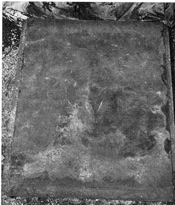
Fig. 10. The 9 ft. By 7 ft. Deck Plate After Removal of the 1\frac{1}{2} -in. Surfacing. Note Absence of Any Corrosion After 4\frac{1}{2} yr., Due to Cracking; and Also the Very Considerable Corrosion Where the Mastic Asphalt Had Not Adhered Properly Over the Front and Centre Portions of the Plate.
