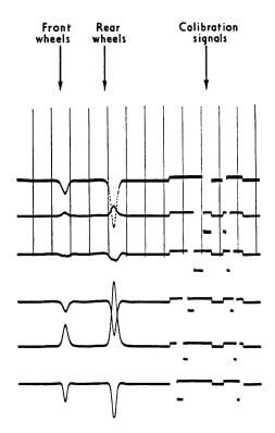
Fig. 14. Dynamic Strain Record. Vehicle Travelling at Creep Speed (About 3 mile/h).
