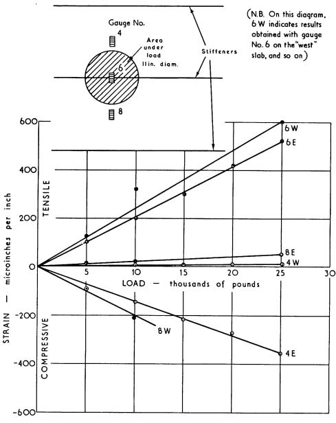
Fig. 12. Results of Static Tests on the Bare Steel Plate With Centre of Load Over Gauge No. 6.
