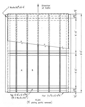
Fig. 1. Deck Panels for First Surfacing Test.
