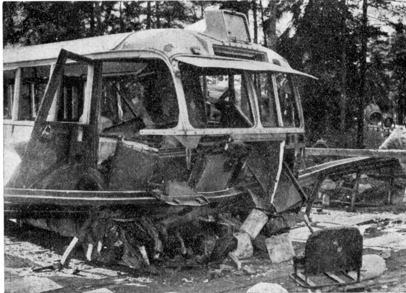
FIG. 8. The Stockholm City's parapet reinforced by welded-on flat bars on a level with the hand-rail. Bus speed just before collision 45 \text{ km/h} .
