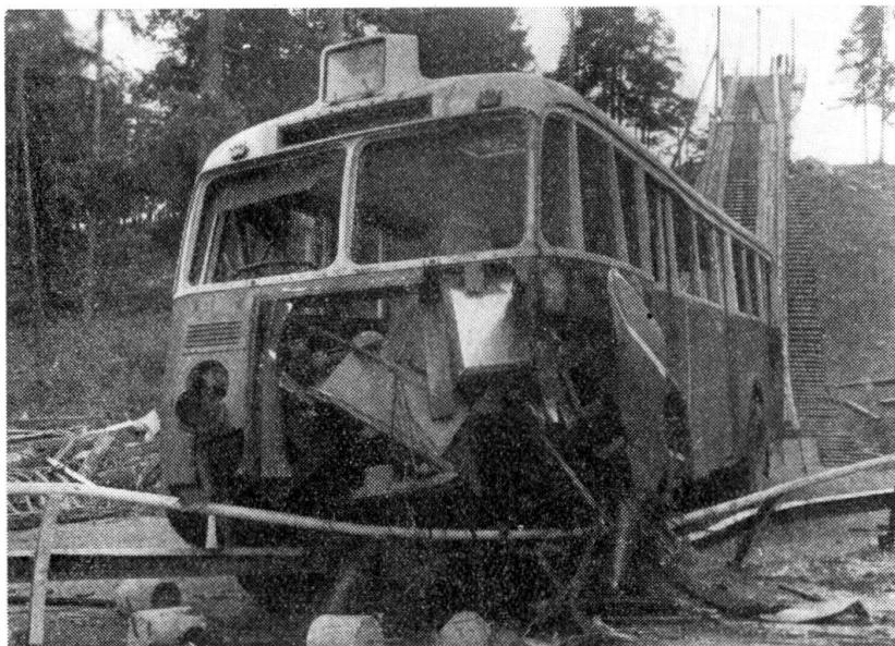
FIG. 11. Warding off parapet between roadway and cycle track after impact at an angle of 45°. Bus speed just before collision 48 km/h.
