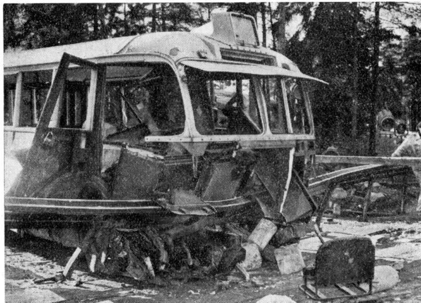
FIG. 8. The Stockholm City's parapet reinforced by welded-on flat bars on a level with the hand-rail. Bus speed just before collision  $45 \text{ km/h}$ .
