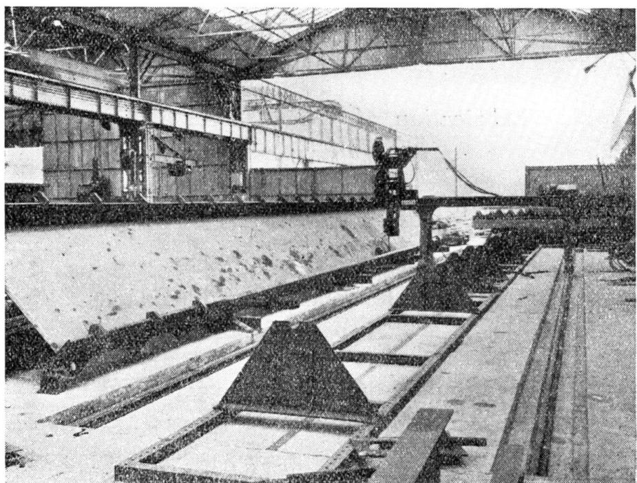
FIG. 1. Welding the web to a flange in a Fusarc automatic welding machine. Note long uninterrupted run attained by adding the stiffeners afterwards
