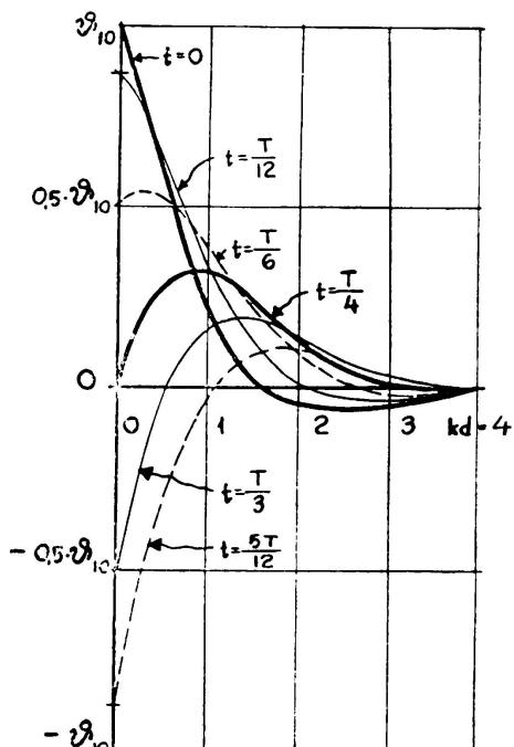
FIG. 8. Temperature conditions for variable surface temperature.
