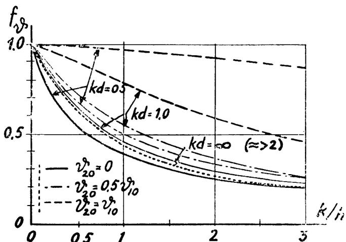
FIG. 10. Amplitude of the surface temperature  $\mathcal{V}_{10}$  if the amplitude of the surrounding air is  $\mathcal{V}_{ao}$
