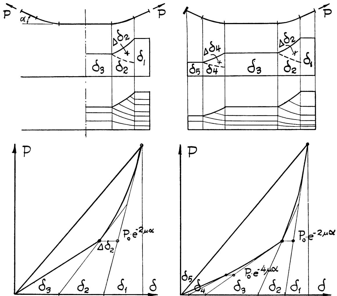
FIG. 4. Curves corresponding to fig. 1 d for cables with straight middle parts.
