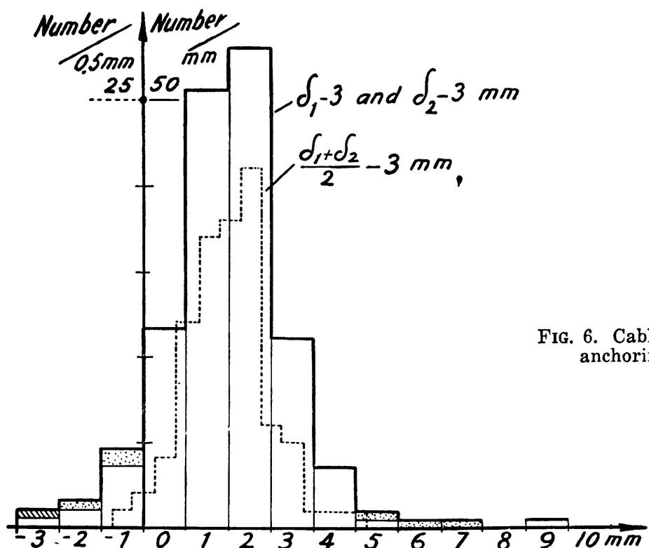
FIG. 6. Cable slip at anchorings.
