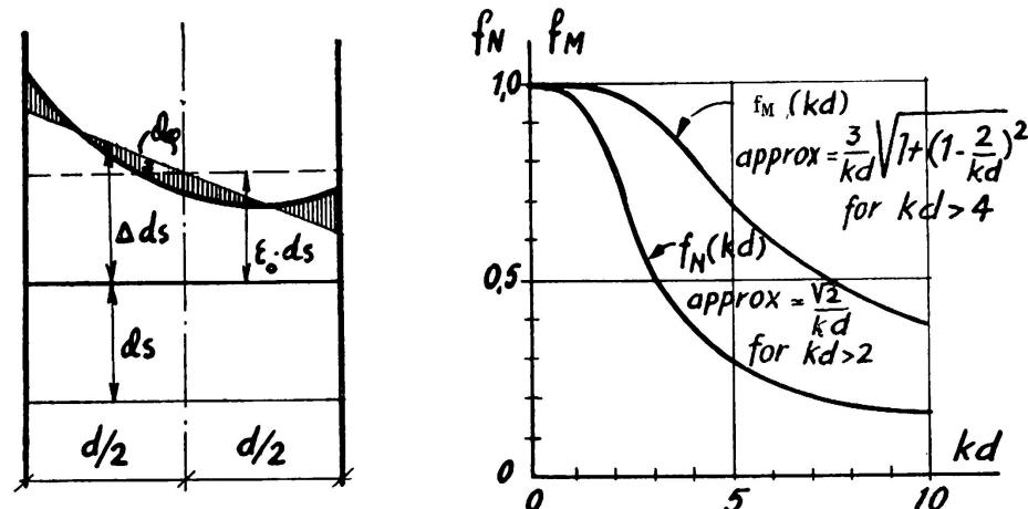
FIG. 9. Length variation and bending of a slab for variable surface temperature. Max. value of the mean temperature  $\mathcal{V}_{mo} = \frac{\mathcal{V}_{10} + \mathcal{V}_{20}}{2}$ .  $f_M(kd)$
