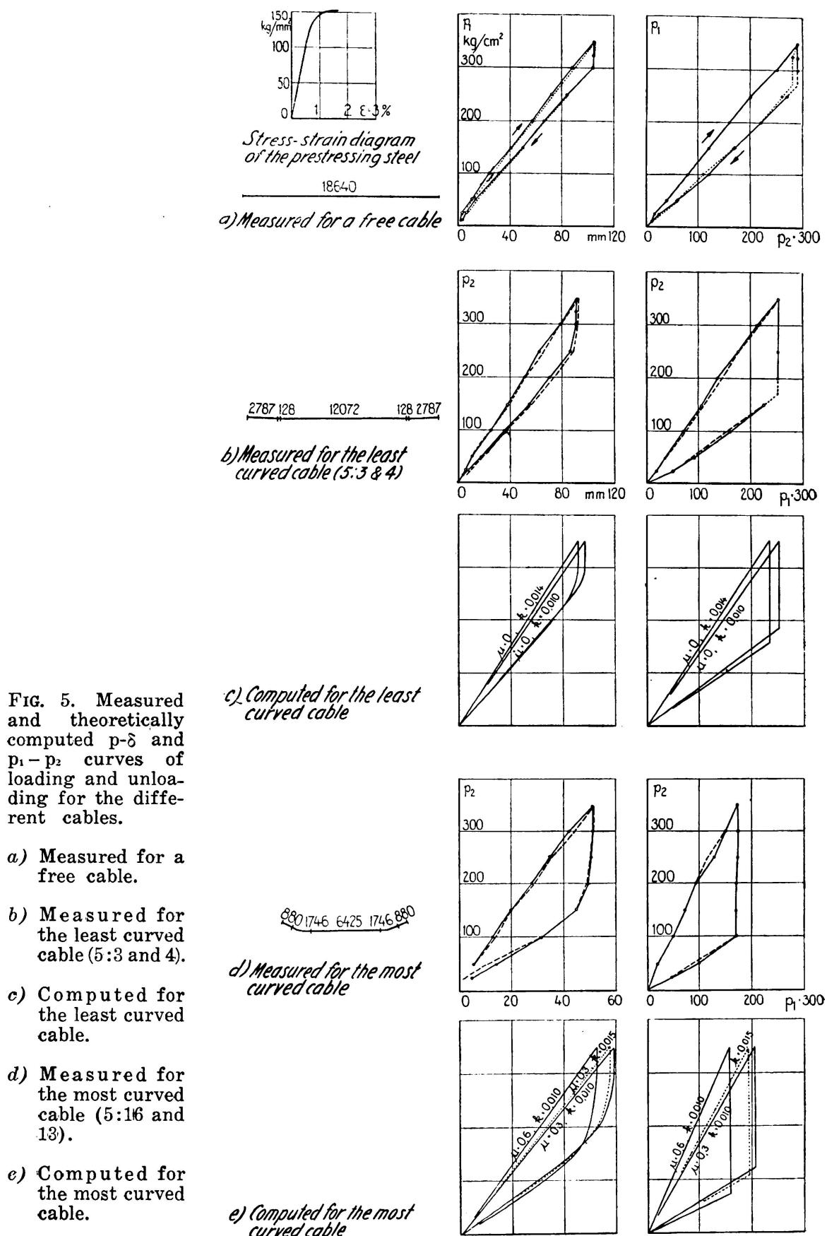
for jack 2. The cables consist of 12 ø 5,0 mm and the jack's piston area is 81,07 cm<sup>2</sup>.
