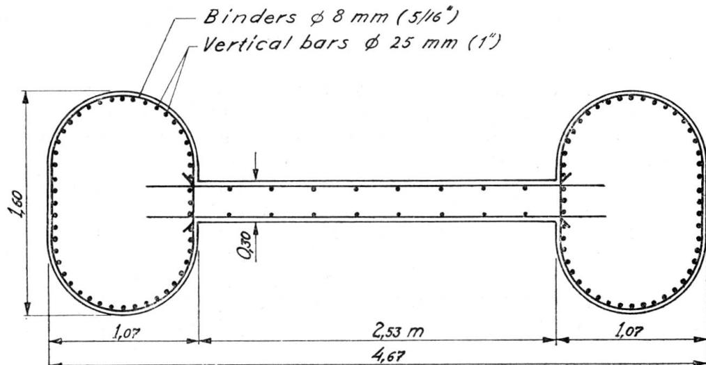
FIG. 2. Cross section of an abutment column
