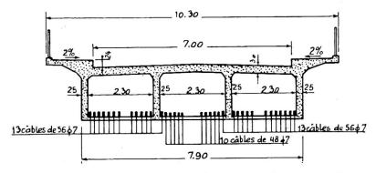
Fig. 15. Bridge over the Meuse at Sclayn in prestressed concrete—Cross-section
