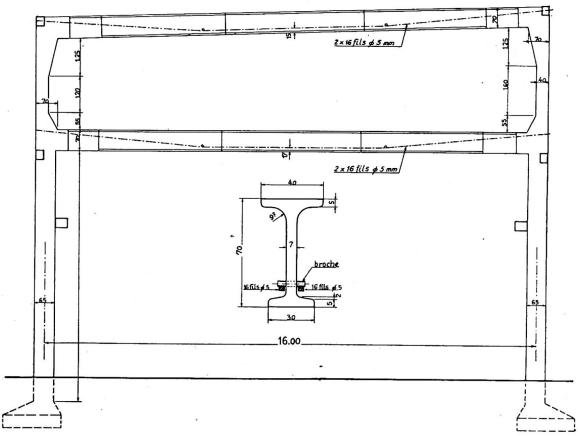
Fig. 6. Factory at Machelen. Depôt—Cross-section
