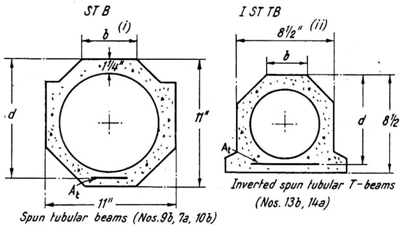
TESTS ON SPUN CONCRETE SPECIMENS
