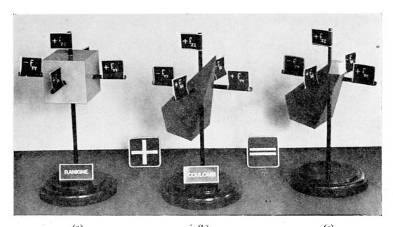
(b) Fig. 7. Space models representing theory of failure for reinforced concrete.  $(f_{xx}, f_{yy}, \text{ and } f_{zz})$  are the three principal stresses, the positive sign denoting tension)
