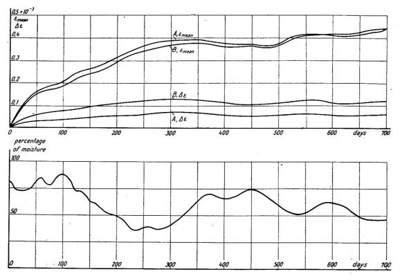
Fig. 7(a). Average shrinkage and difference in shrinkage  $\Delta \epsilon$  between the top and bottom surfaces observed in the shrinkage tests on beams made in accordance with Table III. Consistency of concrete: 11 degrees VB
