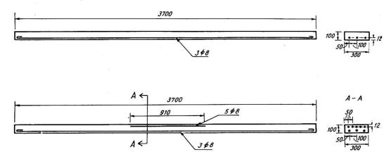
Fig. 2. Dimensions and reinforcement of the beam specimens used in the shrinkage tests
