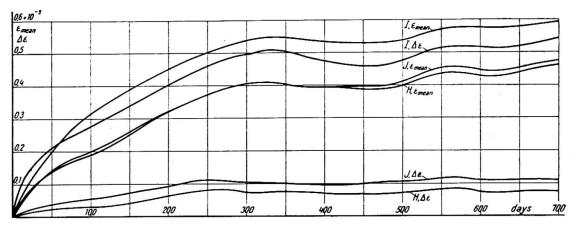
Fig. 7(c). Average shrinkage and difference in shrinkage  $\Delta\epsilon$  between the top and bottom surfaces observed in the shrinkage tests on beams made in accordance with Table III. Consistency of concrete—slump test: 9.0 cm.
