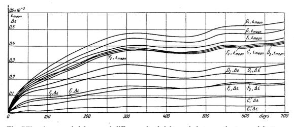
Fig. 7(b). Average shrinkage and difference in shrinkage  $\Delta\epsilon$  between the top and bottom surfaces observed in the shrinkage tests on beams made in accordance with Table III. Consistency of concrete: 5·2 degrees VB. Slump test: 2·3 cm.
