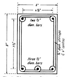
Fig. 4. Dimensions of test specimens
