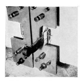
(b) Detail of mechanical tensometers
