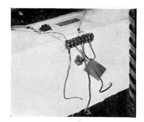
(c) Detail of electrical resistance strain gauges
