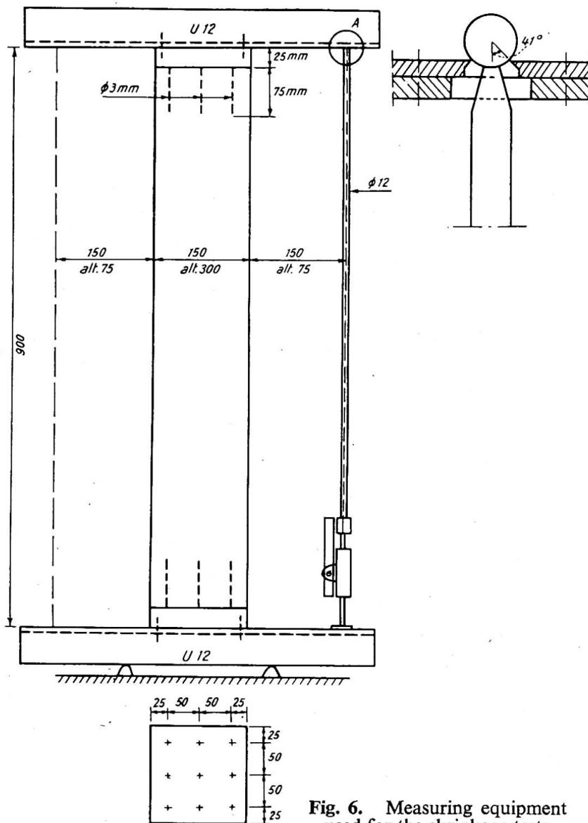
Fig. 6. Measuring equipment used for the shrinkage tests
