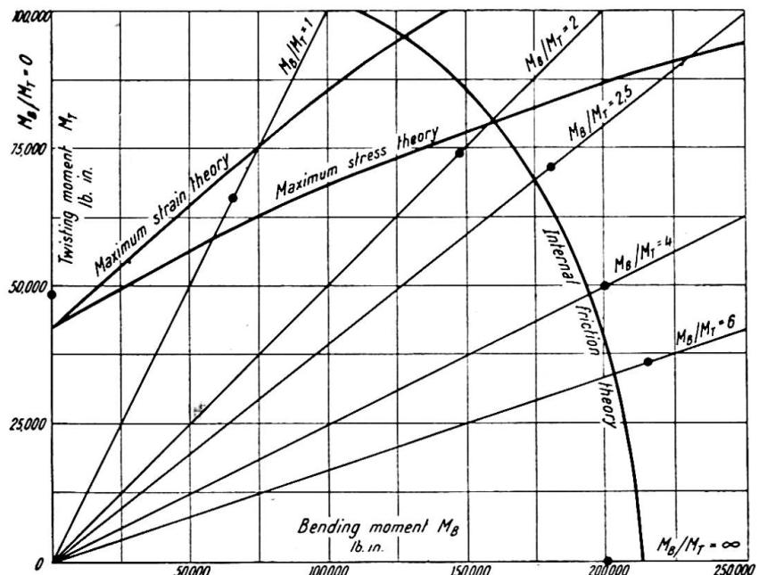
Fig. 6. Bending moments and twisting moments at the breakdown of elastic action. Experimental results ●
