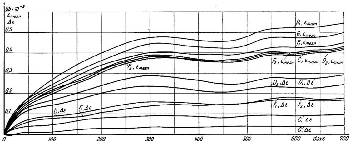
Fig. 7(b). Average shrinkage and difference in shrinkage  $\Delta\epsilon$  between the top and bottom surfaces observed in the shrinkage tests on beams made in accordance with Table III. Consistency of concrete: 5.2 degrees VB. Slump test: 2.3 cm.
