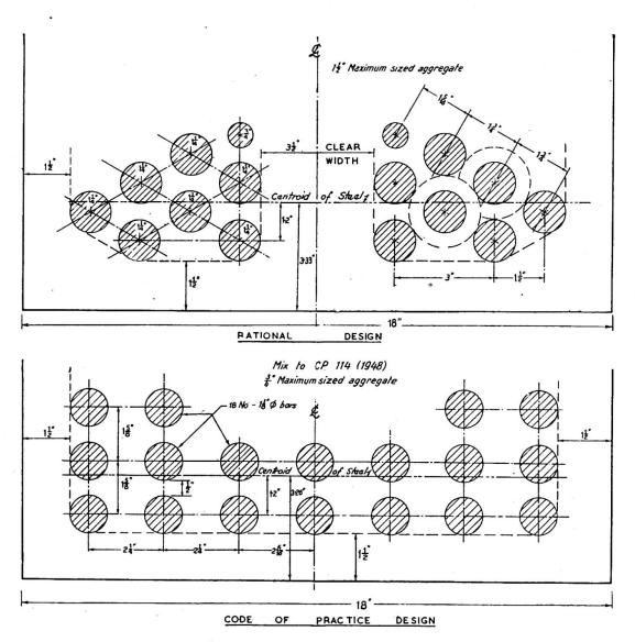
Fig. 4. The comparison of beam design methods
