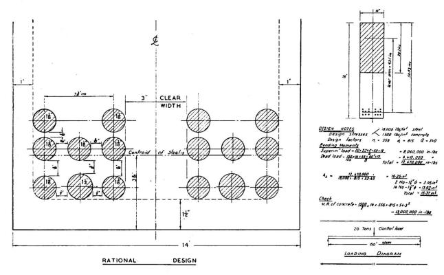
Fig. 3(a). The comparison of beam design methods
