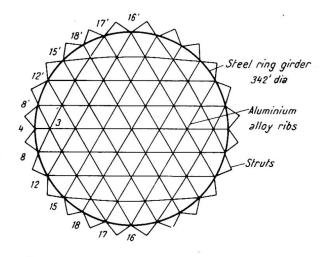
a) Schematic plan view of dome
