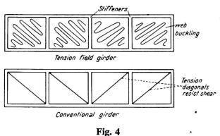
main difference is that the tension field beam is of very thin sheet-metal which is permitted to wrinkle or buckle under shear stress caused by the load. The wrinkled web acts like tension diagonals in ordinary open-web trusses, thus creating a "tension field" within the web. The theory of pure tension field beams was first developed and published by Wagner in 1929 and it is therefore also termed the Wagner beam. In this theory it was assumed that the web was
