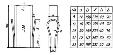
Fig. 3. The dimensions of the tested connectors of type VII
