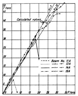
Fig. 8. The total shear force T as a function of the load P
