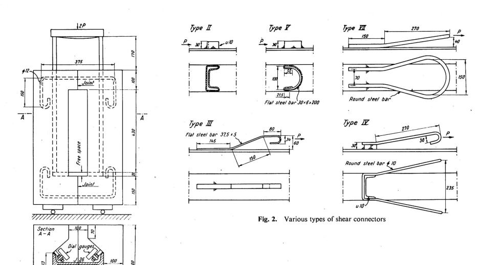
Fig. 1. Test specimen for testing shear connectors
