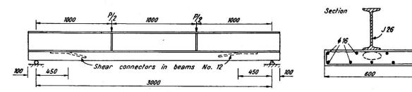
Fig. 10. Test beams No. 12
