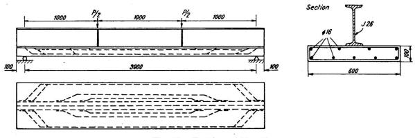
Fig. 11. Test beams No. 18
