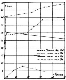
Fig. 9. Relation between the total shear force T and the slip e between steel and concrete
