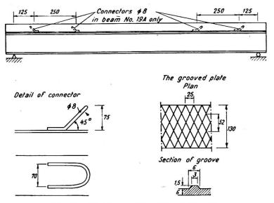
Fig. 5. Test beams No. 14 and No. 19
