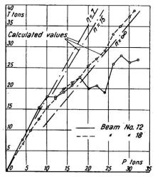
Fig. 13. The total shear force T as a function of the load P
