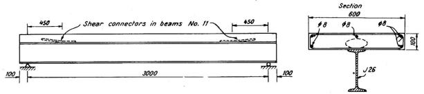
Fig. 4. Test beams No. 11
