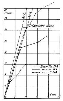
Fig. 7. The deflection δ at the centre of beams No. 13A, No. 14A and No. 19A as a function of the load P
