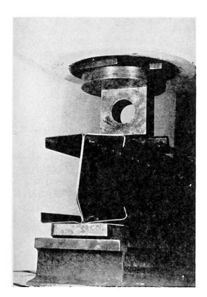
Fig. 7. Web crushing under concentrated loads
