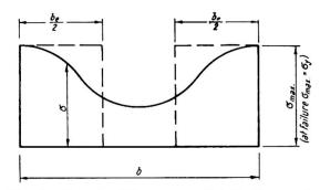
Fig. 2. Post-buckling stress distribution and effective width of stiffened compression plate
