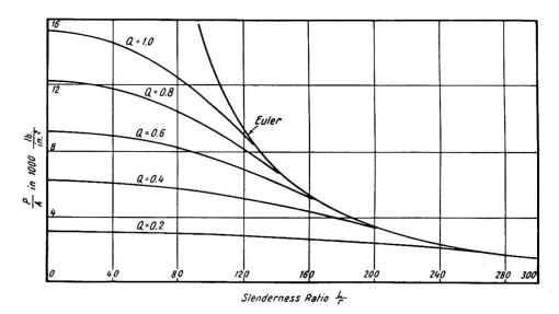
Fig. 6. Permissible column design stresses (yield point=33,000 psi.)
