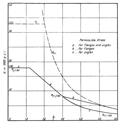
Fig. 5. Permissible design stresses for unstiffened compression elements
