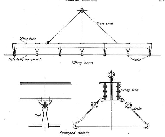
Fig. 2. Typical plate lifting beam
