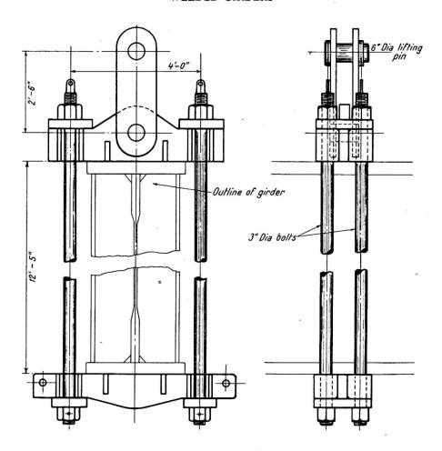
Fig. 11. Lifting cradle for 100-ton girder
