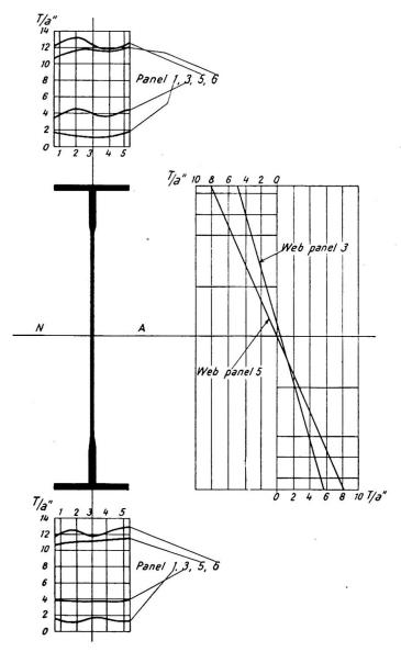
Fig 4. Tests on model girder bending stresses in flanges and web load 75 tons Note: For T/a'' read tons/in.<sup>2</sup>
