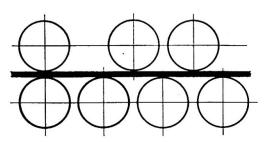
Fig. 1. Arrangement of rolls. Roller levelling machine
