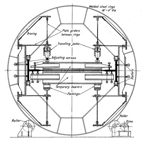
Fig. 7. Cross section through manipulator
