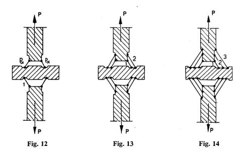
It is assumed that a small portion of the material in the adjoining sections will yield with the rest. The non-yielding parts of these adjoining sections may then be regarded as having  $\sim$  rigidity.
