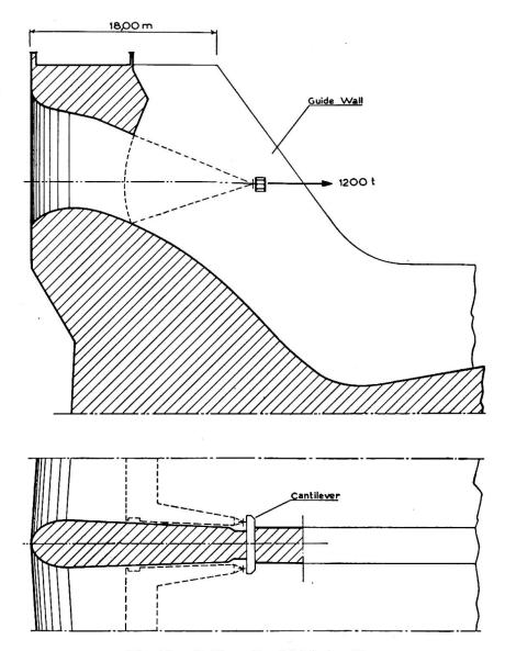
Fig. 18. Guide walls of Mabubas Dam
