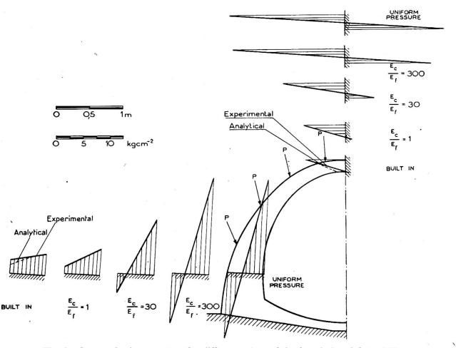
Fig. 4. Stresses in the prototype for different values of the foundation deformability
