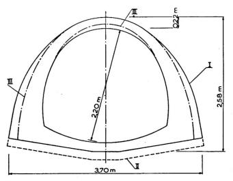
Fig. 1. Cross-section of the aqueduct
