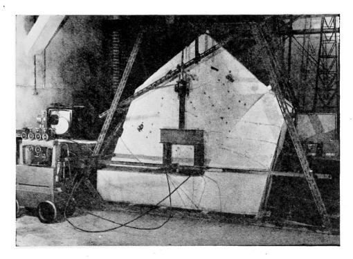
Fig. 21. Reinforced-concrete model to a scale of 1/10
