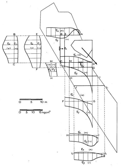
Fig. 17. Normal stress transferred to the prototype
