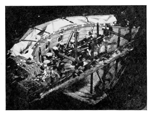
Fig. 7. Model to a scale of 1/300 of a 130 m. high arch dam and its foundations. It was built from plaster diatomite mix and electric strain gauges were used for strain measurements
