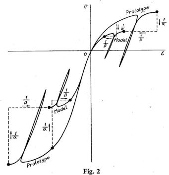
stresses which bring about failure of the parallelepiped. It will be necessary therefore that in the curves of fig. 2 the ultimate strengths of homologous materials be in the relation of  $1/\alpha$  and that they correspond to strains in the relation of  $1/\beta$ .
