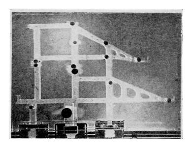
Fig. 11. Photograph obtained in studying a linear structure by the photographic method
