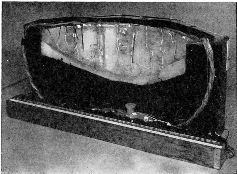
**Fig. 6.** Alkathene model to a scale of 1/200 of a 35 m. high arch dam. The model was subjected to mercury hydro-static pressure and the strains were measured by means of electric strain gauges specially built for use on alkathene
