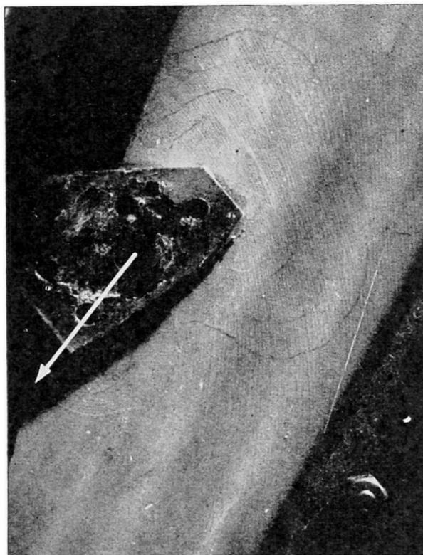
Fig. 9. Application of the brittle coating method to the determination of the isostatics in a spillway guide wall
