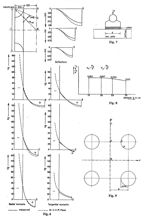
The bending moments  $M_x$  and  $M_y$  in point D (fig. 6) amounted to +25 kg.-cm./cm. and -8 kg.-cm./cm. respectively.
