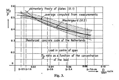
with a rubber packing of 3 mm., higher values of  $M_x/P$  are found. For comparison the values according to the elementary theory of plates <sup>1</sup> and those from the formula of Westergaard <sup>2</sup> are also given. Those of Westergaard also agree well with the test results when the load is concentrated on a very small area.
