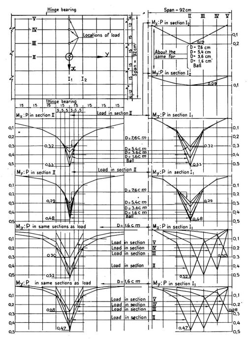
Fig. 2. Moment-load ratio from measured strains
