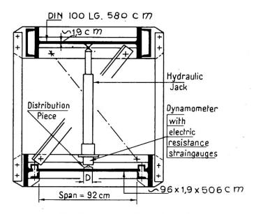
Fig. 1. Cross-section of model
