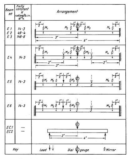
Fig. 10. Summary of tests on fixed-ended beams
