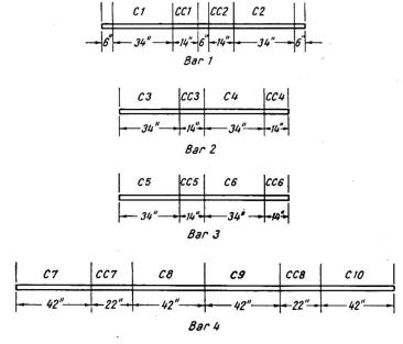
Fig. 1. Division of bars for continuous beam tests
