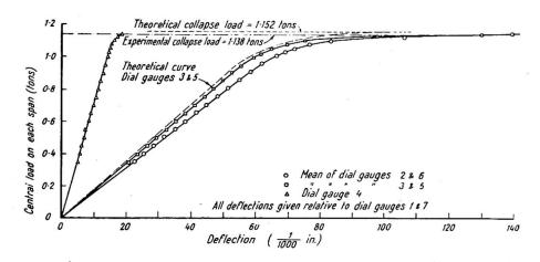
Fig. 6. Load-deflection curves for beam C2
