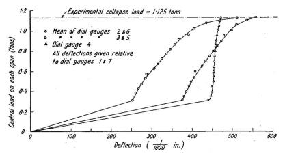
Fig. 5. Load-deflection curves for Beam C1
