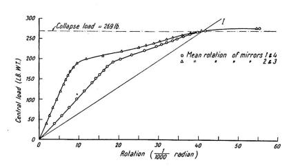
Fig. 14. Load rotation curves for beam E3
