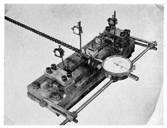
Fig. 11. Arrangement for testing fixed-ended beams
