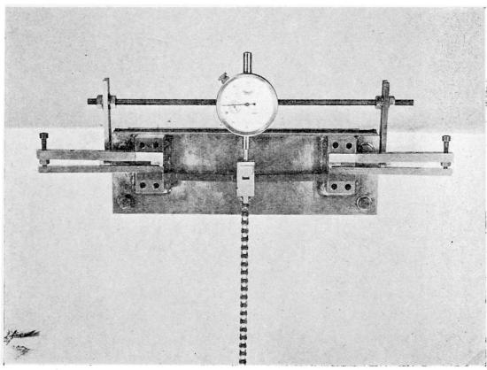
Fig. 12. Method of obtaining reduced end fixity
