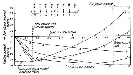
Fig. 9. Theoretical bending moment curves for beam C8
