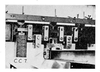
Fig. 4. Arrangement for testing simply supported beams
