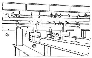
Fig. 3. Arrangement for testing continuous beams
