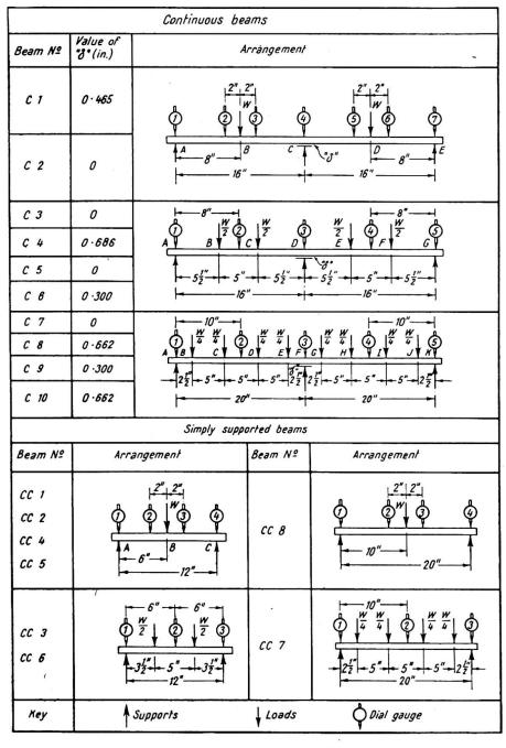
Fig. 2. Summary of continuous beam tests (In beam CC8, for 2" read  $2\frac{1}{2}$ ")
