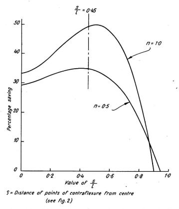
Fig. 3. Economies achieved by continuously varying the section of a fixed-ended beam (uniformly distributed load)
