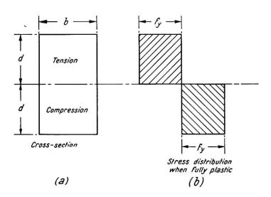
Fig. 1. Fully plastic stress distribution for a rectangular beam
