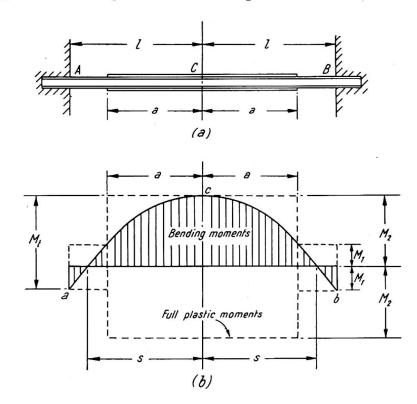
Fig. 4. Bending moment distribution for a beam reinforced at centre only (uniformly distributed load)
