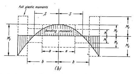
Fig. 8. Bending moment distribution for a beam reinforced at both centre and ends (uniformly distributed load)
