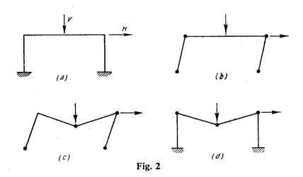
The first part of this paper deals with methods for the exact determination of the quantities required (location of the hinges, values of collapse loads, etc.); the second part presents methods for determining upper and lower bounds on the loads, it being possible to make these bounds as close as is considered necessary. The third part applies the ideas to space frames, where hinges are formed under the combined action of bending and torsion.
