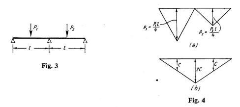
Since the continuous beam system under consideration has one redundancy, the plastic behaviour can be represented as the sum of an equilibrium state and one residual state, which may be taken as the two bending moment distributions in fig. 4. The continued inequality (2) may be written for the three critical sections:
