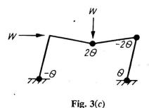
For each mechanism it is possible to calculate a corresponding value of W by applying the principle of virtual work in the special form that the virtual work done by the applied loads during a small displacement of the mechanism is equal to the virtual work absorbed in the plastic hinges. Considering the mechanism of fig. 3(a), for example, it is seen that during the small mechanism dis-
