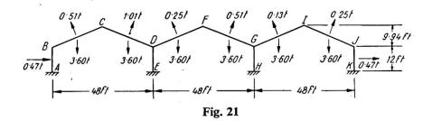
distributed, and the vertical loads of 3.60 tons on each rafter member are due to dead and superimposed loads, the remaining loads being wind loads. In the first instance, it will be assumed that all the members of the frame are of the same cross-section, with a fully plastic moment  $M_p$ .
