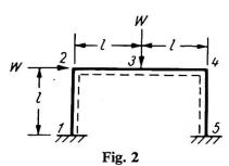
hinge rotations are all shown in terms of a single parameter  $\theta$ . For reference, the signs of the plastic hinge rotations are also given, although in the technique to be described there is no need to take account of these signs. The sign convention adopted is that a hinge rotation is positive if the hinge is opening when viewed from inside the frame.
