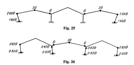
of  $M_p$  greater than 20.6 tons-ft. The mechanism of fig. 25 is thus the actual collapse mechanism, subject to alterations due to the occurrence of plastic hinges at positions other than at the ends and centres of the members. A statical check will now be made which will also serve to indicate such alterations in the position of the plastic hinges.
