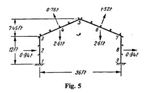
case in which only the dead and superimposed loads are acting, and to a load factor of 1.4 for the case in which the wind loads are also acting. Each member of the frame will be taken to have the same cross-section, with a fully plastic moment  $M_p$ .
