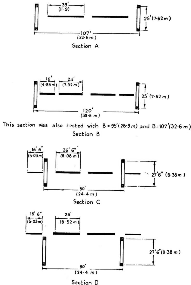
Fig. 3. Main types of bridge sections tested
