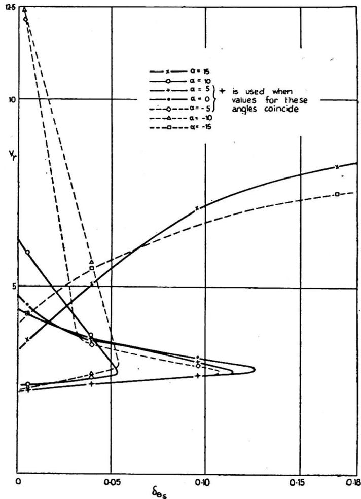
Fig. 4. Influence of damping on the pitching oscillations of the plate girder stiffened section A
