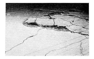
In another test with a 2 000 kilos missile, the observed vertical deformation, without serious damage to the shell, was 25 cm.
