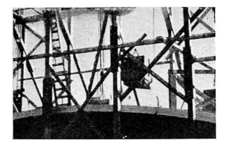
Fig. 3. Impact load on a 9.5 cm reinforced shell roof with a clear span of 14.2 meters. A concrete block weighing 1 000 kgs is released from a height of 3 meters. The picture was taken immediately before the impact.
