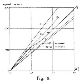
Curve a. Maximum value calculated from cube compressive strength of concrete and ultimate stress of reinforcement bars  $l\sigma = 442 \text{ kg/cm}^2$  and
