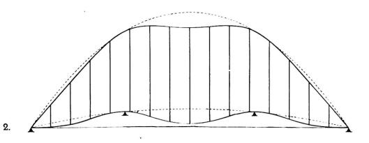
differing from 90 degrees, any effect on the camber, which has been proven in practice, as long as the leading principle is carried out conscientiously namely reaming and riveting both the stiffening girder and the arch in the shape computed for the unstressed condition.
