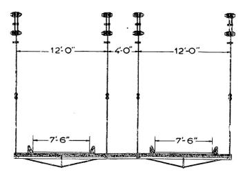
Fig. 1. Cross section of Telford's original deck.
