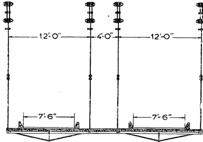
Fig. 1. Cross section of Telford's original deck.
