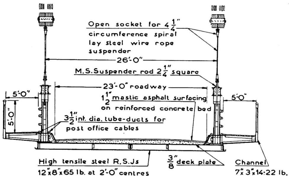
Fig. 2. Cross section of deck as reconstructed in 1940.
