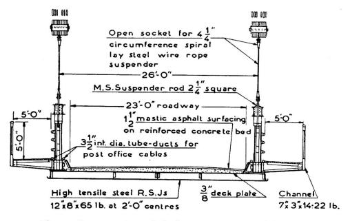
Fig. 2. Cross section of deck as reconstructed in 1940.
