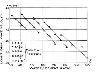
Fig. 6. Longitudinal wave velocity in concrete at an age of 7 days.
