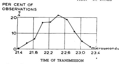
Fig. 2. Distribution of transmission times in concrete cubes.
