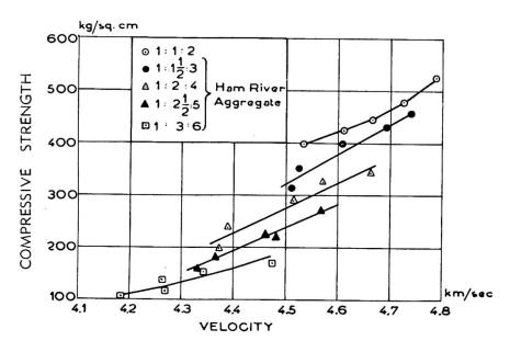
Fig. 8. Relation between the longitudinal wave velocity and the compressive cube strength.
