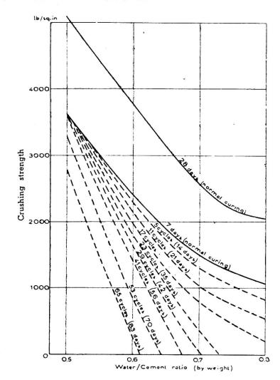
Fig. 2. Relation between crushing strength and water-cement ratio for various numbers of freezing and thawing cycles.
