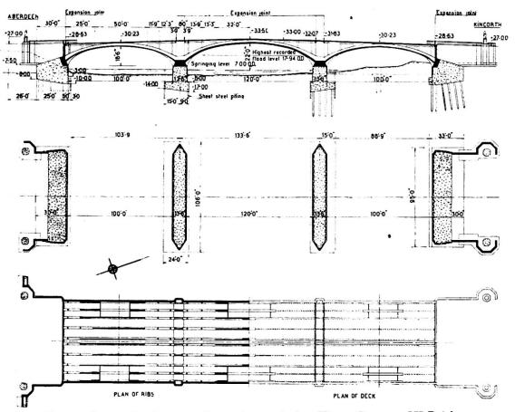
Fig. 1. General plans and sections of the King George VI-Bridge.
