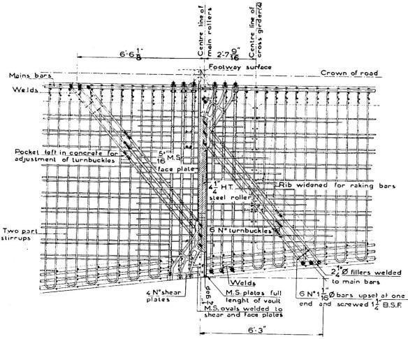
Fig. 6. Centre span (expansion joint details).
