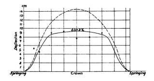
Fig. 7. Deflection at the freely suspended centering some hours before the collapse.
