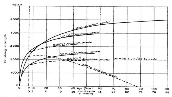
Fig. 8. Effect of addition of aluminium powder on the frost resistance of concrete.
