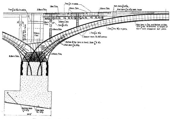
Fig. 5. Details of construction of the river span.
