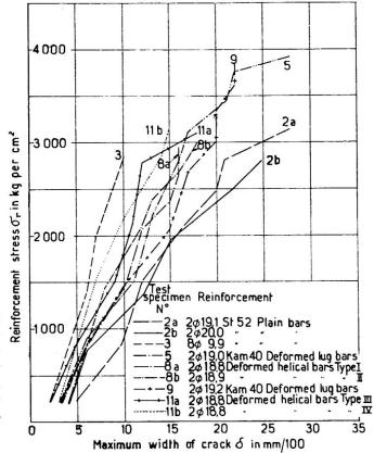
Fig. 4. Width of largest crack δ as a function of the reinforcement stress σ, during the third application of load to ten test beams differing in diameter of reinforcement bars (Nos. 2b, 2a and 3) and in surface properties of reinforcement bars (Nos. 2a, 2b, 5, 9, 8a, 8b, 11a and 11b).
