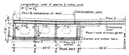
Fig. 5. Half cross section at crown.
