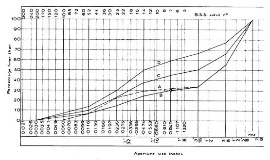
Fig. 5. Grading curves of aggregates.
