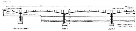
Fig. 3. Longitudinal section through box girder.
