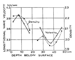
Fig. 5. Longitudinal wave velocity and density at various depth in a road slab.
