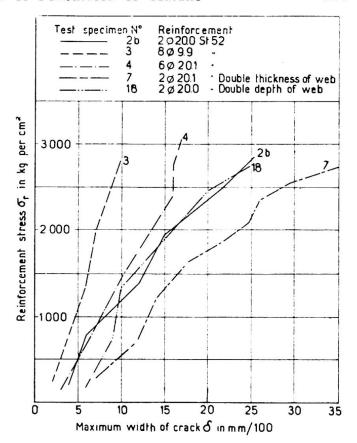
Fig. 2. Width of largest crack & as a function of the reinforcement stress of during the third application of load to five test beams differing in diameter of reinforcement bars (Nos. 2b and 3), ratio of reinforcement (Nos. 2b and 4), thickness of web (2b and 7), and depth of web (2b and 18).
