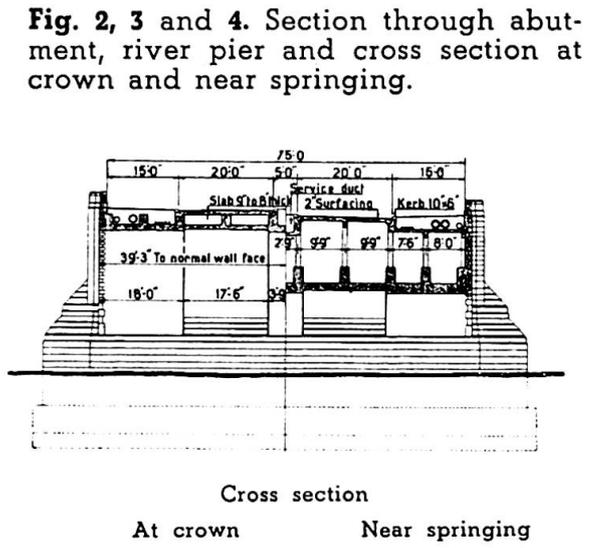
Fig. 2, 3 and 4. Section through abutment, river pier and cross section at crown and near springing.
