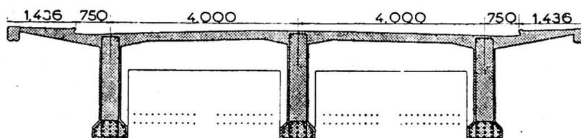
Fig. 16. Cross-section with the freely suspended tie-roads.
