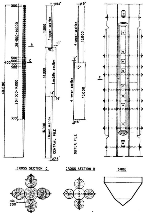
Fig. 10 (above). Pile of timber.
