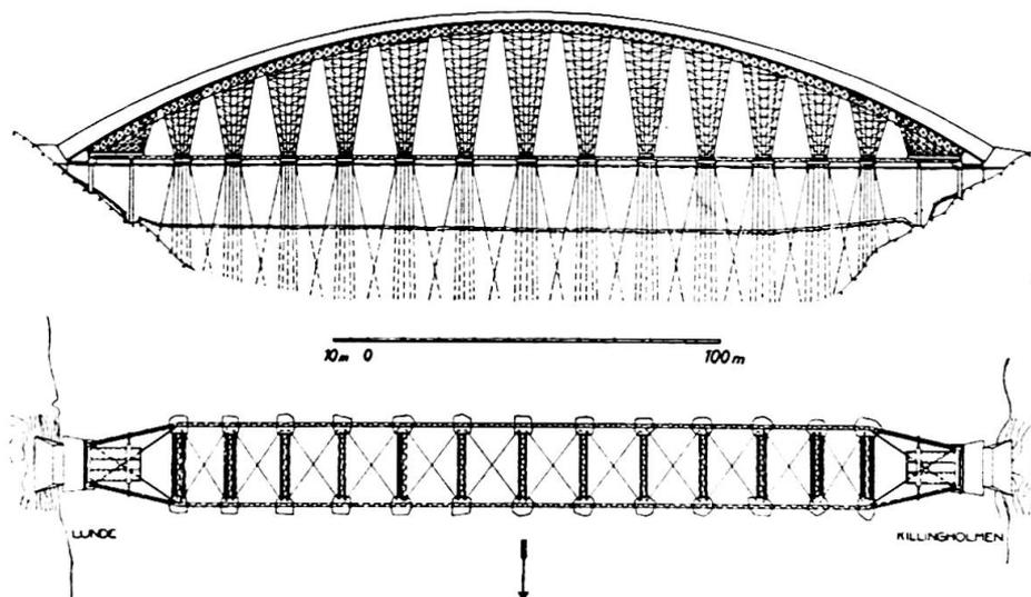
flange at the crown due to the normal thrust from dead load, temperature and increased moisture content of the timber was  $69 \text{ kg/cm}^2$ . From the moment due to the bending of the planks, reduced by 33 % by creeping, and the eccentricity of the normal thrust in the bent flange the total bending stress was calculated to be  $32 \text{ kg/cm}^2$  corresponding to an eccentricity of the normal thrust of 1.56 cm.
