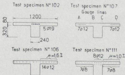
Fig. 5. Cross-section and reinforcement of four specimens used in tests regarding formation of cracks in beams subjected to negative moments.
