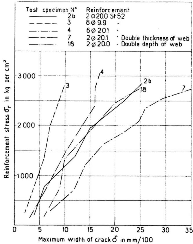
**Fig. 2.** Width of largest crack  $\delta$  as a function of the reinforcement stress  $\sigma_r$  during the third application of load to five test beams differing in diameter of reinforcement bars (Nos. 2b and 3), ratio of reinforcement (Nos. 2b and 4), thickness of web (2b and 7), and depth of web (2b and 18).
