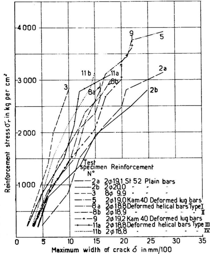
**Fig. 4.** Width of largest crack  $\delta$  as a function of the reinforcement stress  $\sigma_r$  during the third application of load to ten test beams differing in diameter of reinforcement bars (Nos. 2b, 2a and 3) and in surface properties of reinforcement bars (Nos. 2a, 2b, 5, 9, 8a, 8b, 11a and 11b).
