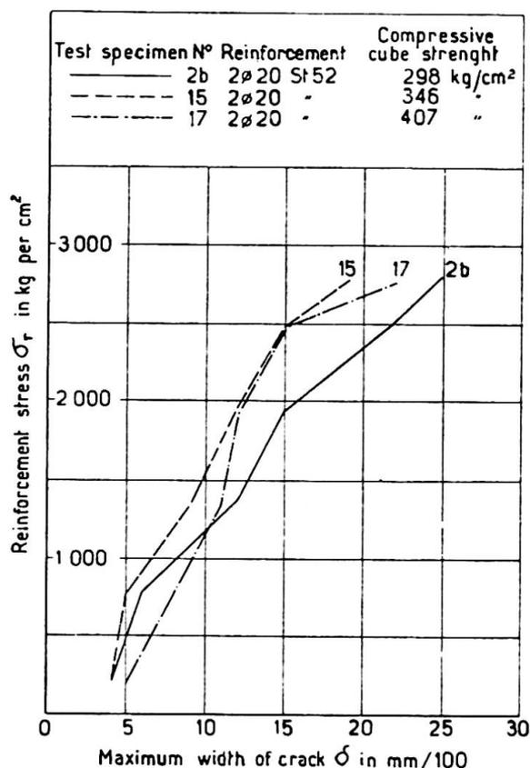
**Fig. 3.** Width of largest crack  $\delta$  as a function of the reinforcement stress  $\sigma_r$  during the third application of load to three test beams differing in concrete strength.
