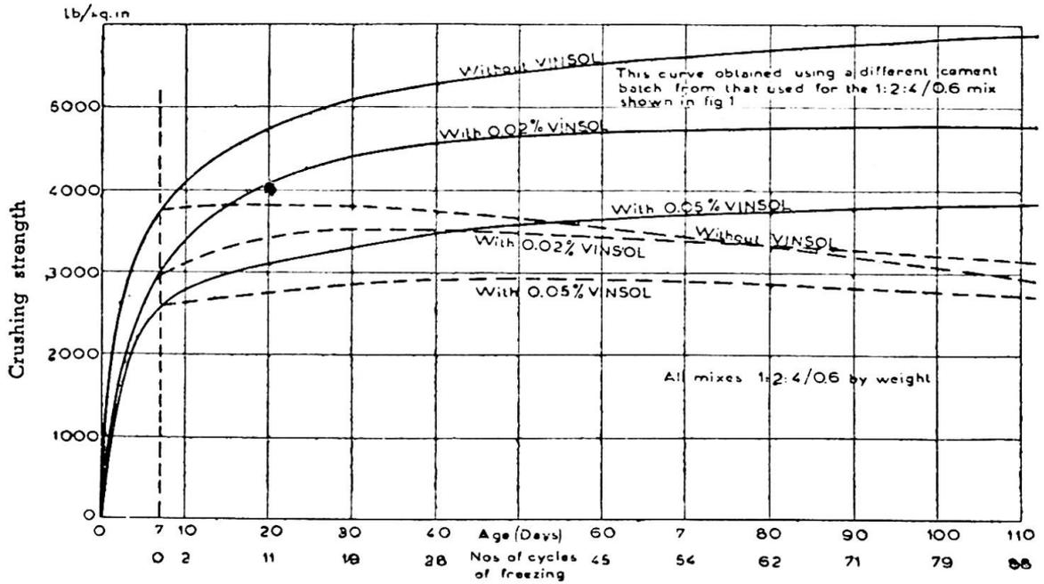
Fig. 7. Effect of addition of Vinsol resin on the frost resistance of concrete.
