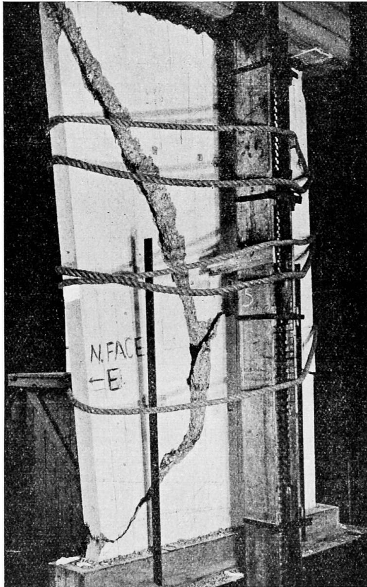
**fig. 1.** View of wall 1B4 after failure.
