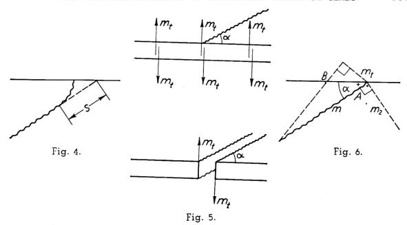
the case (fig. 4), but only quite close to the edge do the cracks suddenly turn so as to be at right angles to it.
