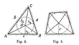
$h_a = h_b = h_c = r$ , where r is the radius of the inscribed circle. The breaking moment is  $m = 1/6 wr^2$ , where w is the ultimate load.
