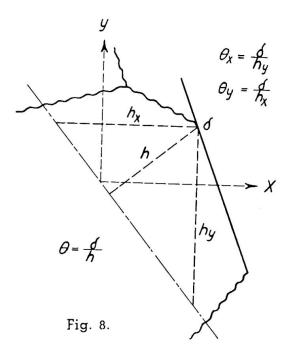
tors are resolved into components along two axes which are at right angles to each other, we get the expression  $(M\theta) = M_x \theta_x + M_y \theta_y$ . The rotation is determined, for instance, by the sinkings as shown in figure 8.
